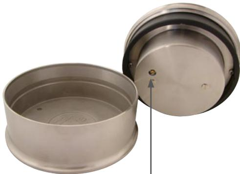
Adjusting screw for calibrating the barometer.
